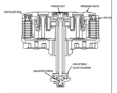
**28.** Using the long end of a 4mm Allen key, turn the adjuster screw clockwise until it stops under moderate pressure. You are trying to feel for the point at which the throwout will start to lift the pressure plate. This is the "starting point".
