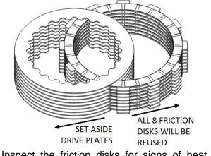
Inspect the friction disks for signs of heat or wear. Replace if they are burnt or worn.
