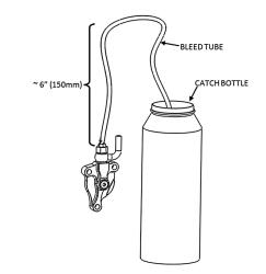
**23.** Pump the clutch lever 3-5 times then hold it against the bar/grip.
