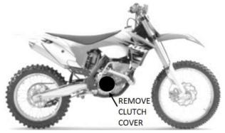
2. Remove the OEM clutch parts named in the following diagram down to the center hub. Leave the thrust washer installed in the basket.
