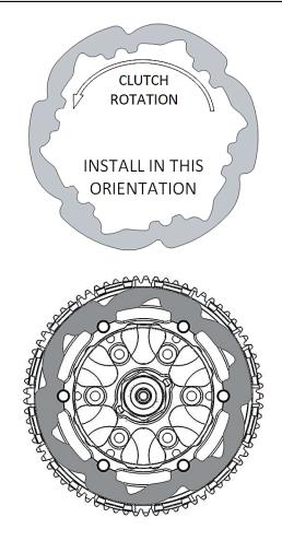
**9.** Install the rest of the clutch pack, noting the number and order of plates shown.
