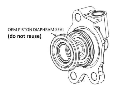
**NOTE:** Some models have a piston diaphragm seal. DO NOT REUSE them if OEM equipped.
