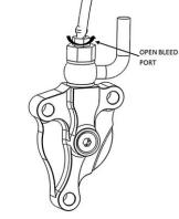
**25.** Slowly release the clutch lever and check the fluid level in the clutch master cylinder.
