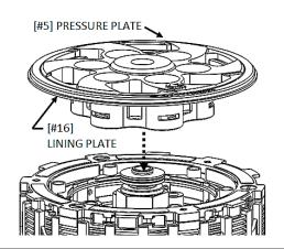
13. Install the Rekluse pressure plate springs and torque the pressure plate bolts.Do not reuse the OEM springs!
