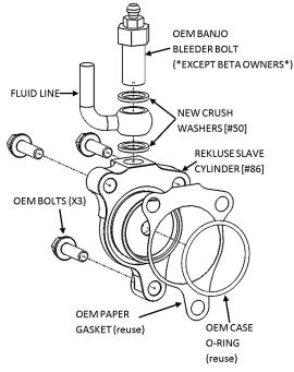
**NOTE:** Some models have a paper gasket and/or O-ring seal. Reuse them if OEM equipped.
