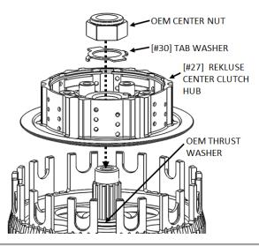
6. Torque the nut to OEM specification, and bend up **both** tabs of the tab washer using channel-lock pliers.
