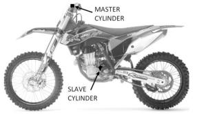
**16.** Starting at the slave cylinder, remove the OEM parts named in the following diagram beginning with the banjo bolt.
