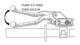
**24.** Using an 8mm wrench, open the bleed port. Air and fluid should come out of the bleed tube. Tighten the bleed port.
