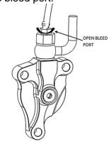
**25.** Slowly release the clutch lever and check the fluid level in the clutch master cylinder.
