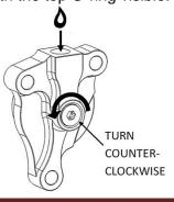
f. Compress the piston until it bottoms out. Repeat the process until there is no longer air escaping from the top port when the piston is compressed.
