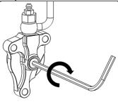
29. Once you have found the starting point, turn the adjuster clockwise 1 full turn plus 5 marks (or "1+5"). This is NOT your final setting, but it is a good reference point for using free play gain to find the correct setting.
