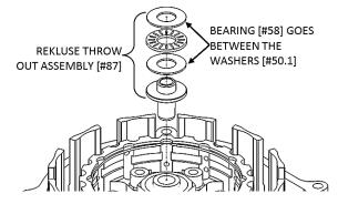
Husqvarna 125cc ('14 and newer) & KTM 125/144/150/200cc ('06 & newer): Install the included throw out spacer onto the OEM throw out.
