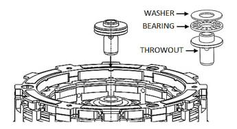
**NOTE**: If you are missing the top washer, it is probably stuck to the backside of your OEM pressure plate.
