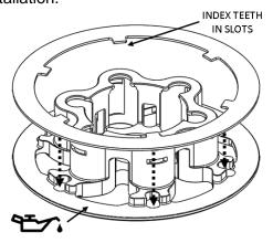
12. Install this pressure plate subassembly.
