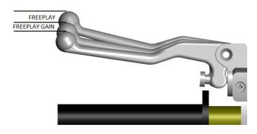
Optimal Free Play Gain yields 1/8" (3mm) of clutch lever movement, measured at the end of the lever. This measurement at the lever correlates to achieving the ideal installed gap.
