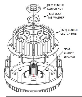
**NOTE**: If the OEM thrust washer is not in place, it is probably stuck to the backside of your OEM center clutch hub.
