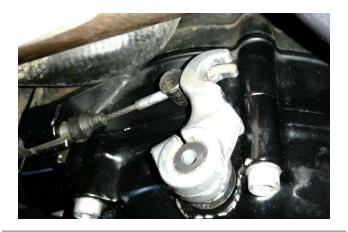
4. Remove the clutch cover bolts and clutch cover.
