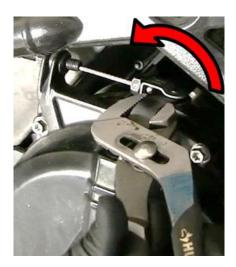
**NOTE:** After you complete the steps in the next section (setting and verifying the installed gap), the actuator arm will rest at nearly 90 degrees to the cable, as shown here.
